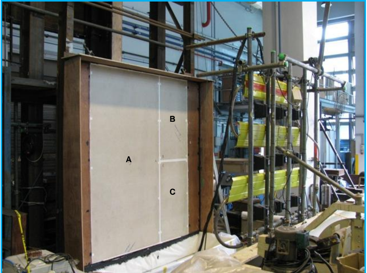
Photo 1: "V-Premium" fibre cement board" mock-up. (Indicated with numbering markings for surface observation before and after test)
